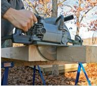
A big blade chops studs with a single cut. Replacing my wormdrive saw's standard blade and housing assembly with a BigFoot version lets me cut with a 10½-in.dia. blade. I gang the sidewall studs together, square the ends, and cut them to the same length in a single pass. A BigFoot attachment costs about \$290 (www.bigfootsaws.com).
