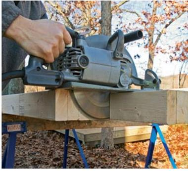
**A big blade chops studs with a single cut.** Replacing my worm-drive saw's standard blade and housing assembly with a BigFoot version lets me cut with a 10¼-in.-dia. blade. I gang the sidewall studs together, square the ends, and cut them to the same length in a single pass. A BigFoot attachment costs about \$290 ([www.bigfootsaws.com](http://www.bigfootsaws.com)).
